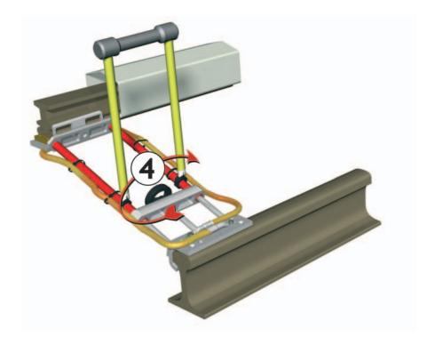
4. The short-circuiter is in place and work on railway can start under safety condition.
