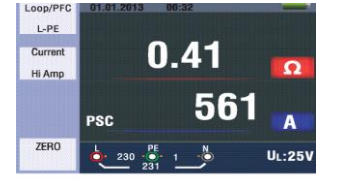
Figure 13 L-N Line Impedance -Measurement completed
