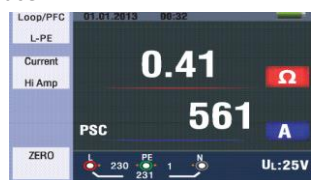
Figure 13 L-N Line Impedance -Measurement completed
