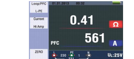
Figure 9 Hi Amp Loop-Measurement finished
