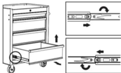
Re-inserting the drawers: pull the slides and slide carrier out until fully extended. Hold the slide on the drawer while aligning it with the slide on the cabinet. Slightly insert one side and repeat for the other side. Slowly push the drawer until it is fully closed to engage the slide. Open and close the drawer to verify proper operation.
