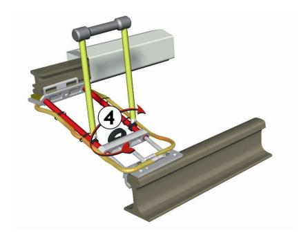
4. The earthing system is in place and work on railway can start under safe condition.
