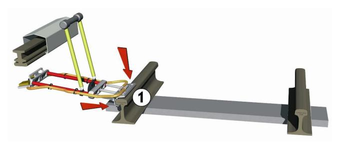
2. Pull up the MT-300/70 device by the handle (2) until the magnet contact blocks and fixes on the current rail (3).
