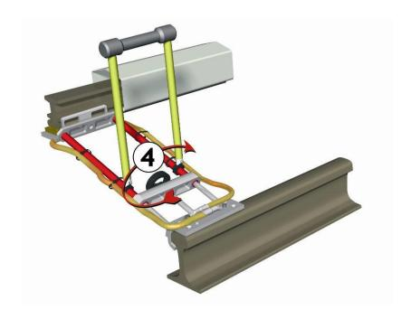
4. The short-circuiter is in place and work on railway can start under safety condition.
