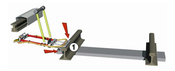
2. Pull up the system by the handle (2) until the magnetized contact block has been fixed on the current rail (3).
